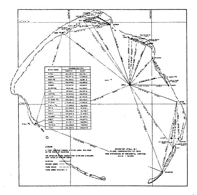
Figure 2-3. 1954 Survey Expansion of Horizontal Control - Eniwetok
