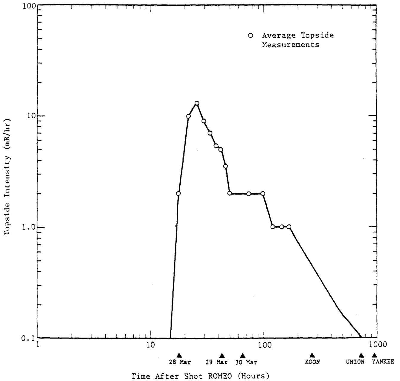
Figure 3.10. Topside intensity on USS MOLALA (ATF-106) following Shot ROMEO.
