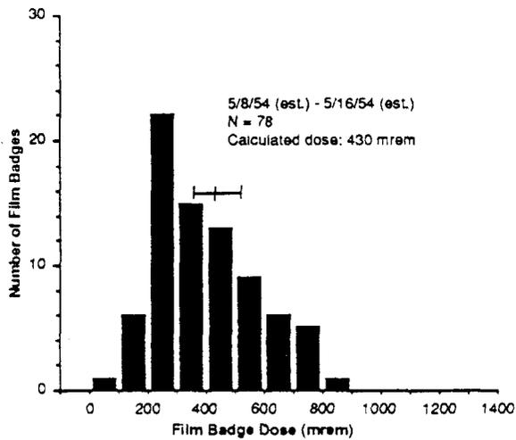
Figure 6.5. Film badge dosimetry for USS MOLALA (ATF-106) (concluded).
