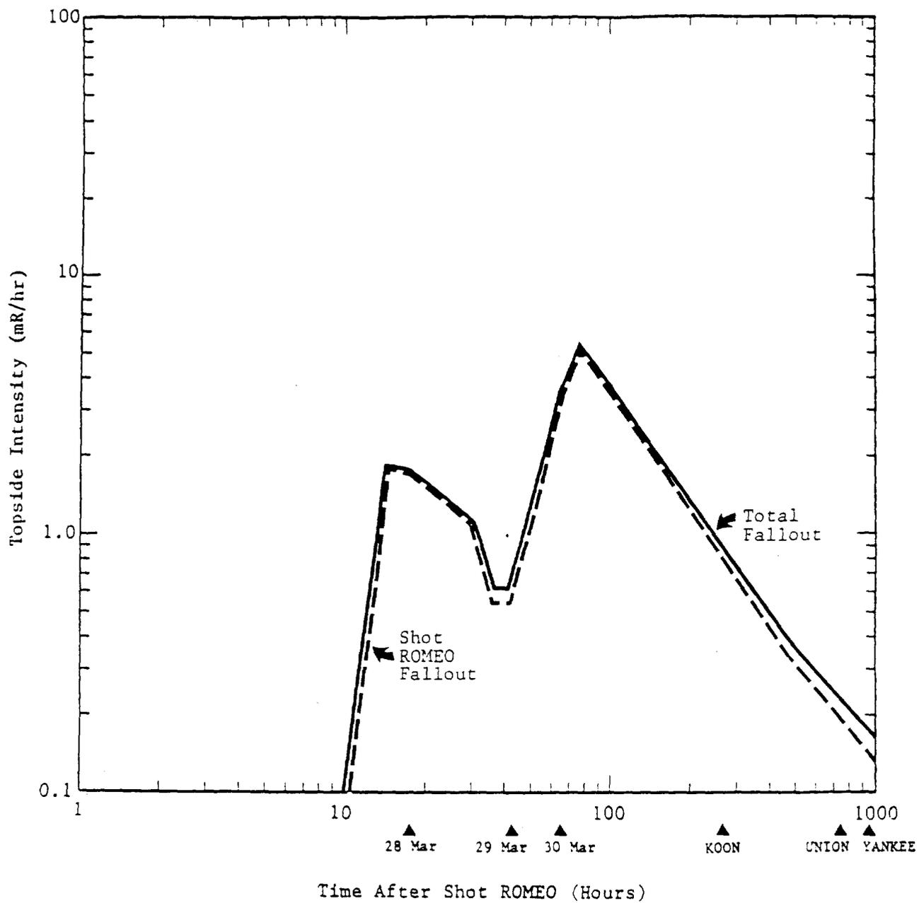
Figure 3.14. Estimated topside intensity on USS PC-1546 following Shot ROMEO.
