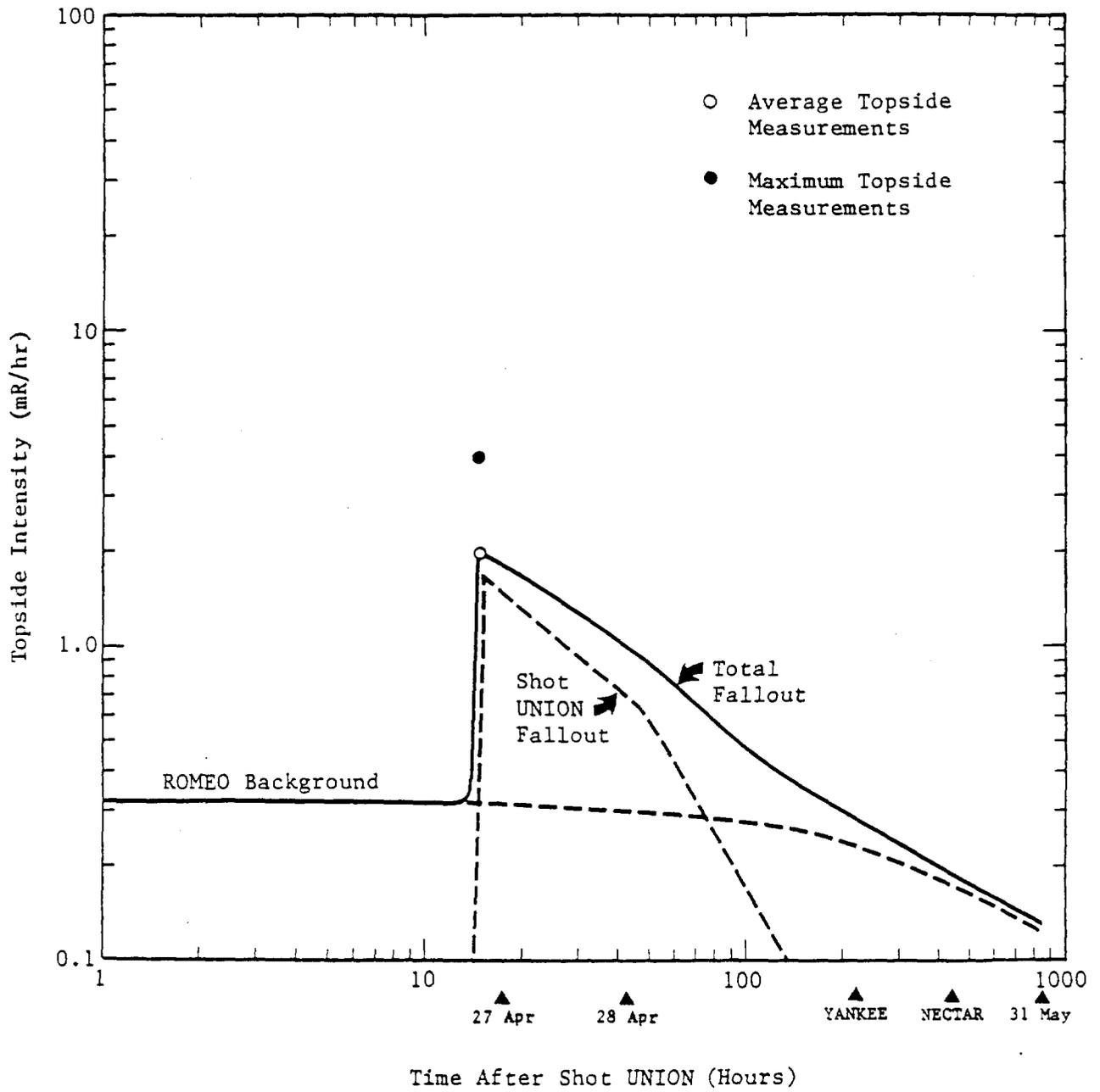
Figure 3.8. Topside intensity on USS MENDER (ARSD-2) following Shot UNION.
