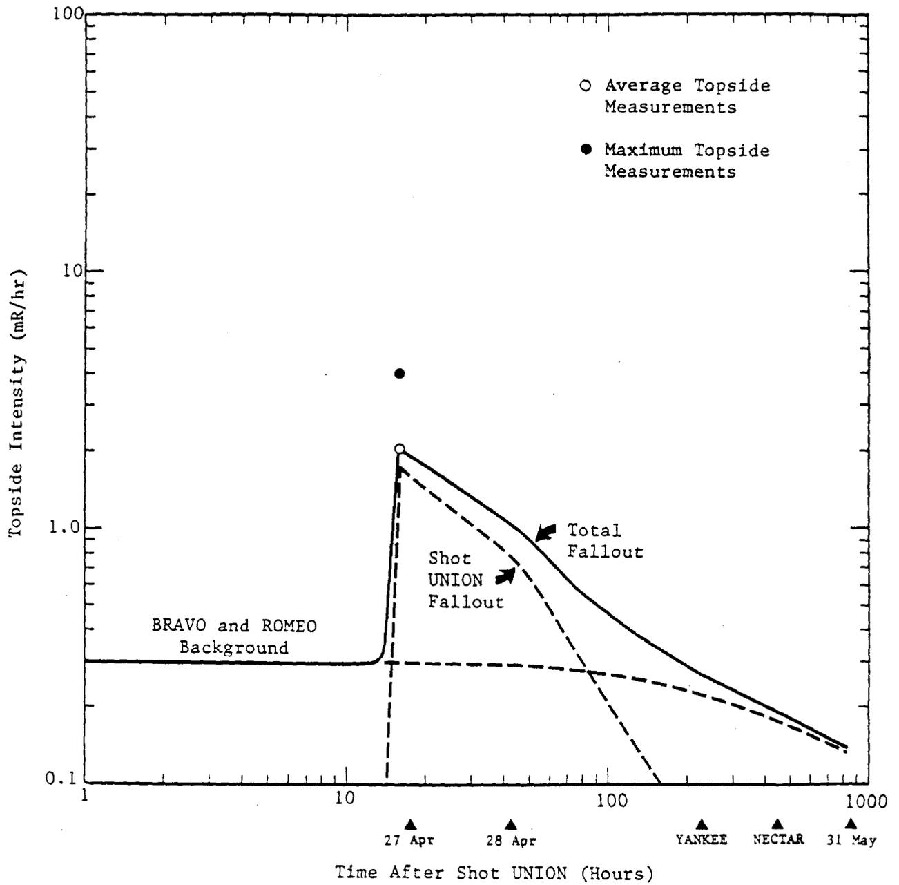
Figure 3.6. Topside intensity on USS COCOPA (ATF-101) following Shot UNION.
