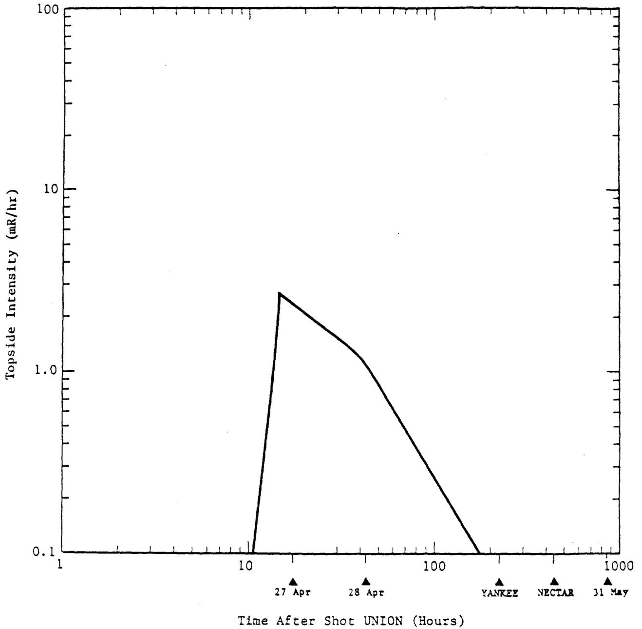
Figure 3.1. Estimated topside intensity on USS RECLAIMER (ARS-42) following Shot UNION.
