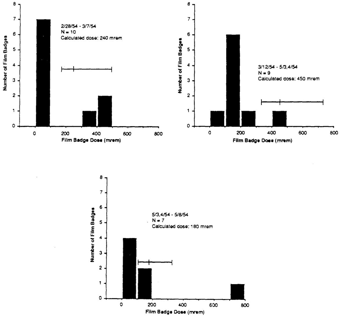
Figure 6.6. Film badge dosimetry for USS TAWAKONI (ATF-114).
