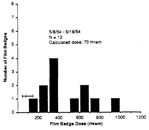
Figure 6.3. Film badge dosimetry for USS COCOPA (ATF-101).
