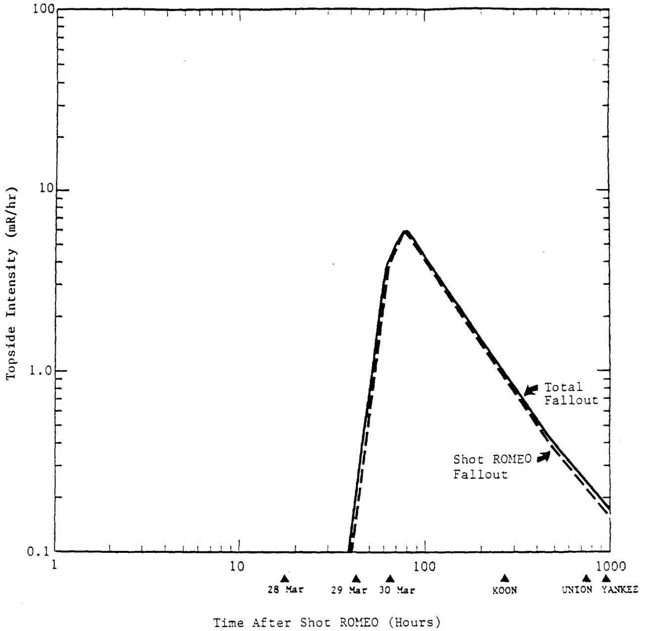
Figure 3.12. Estimated topside intensity on USS TAWAKONI (ATF-114) following Shot ROMEO.
