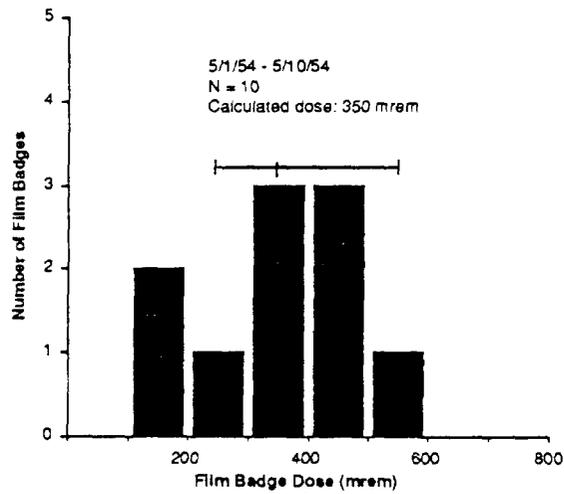
Figure 6.4. Film badge dosimetry for USS MENDER (ARS-2).
