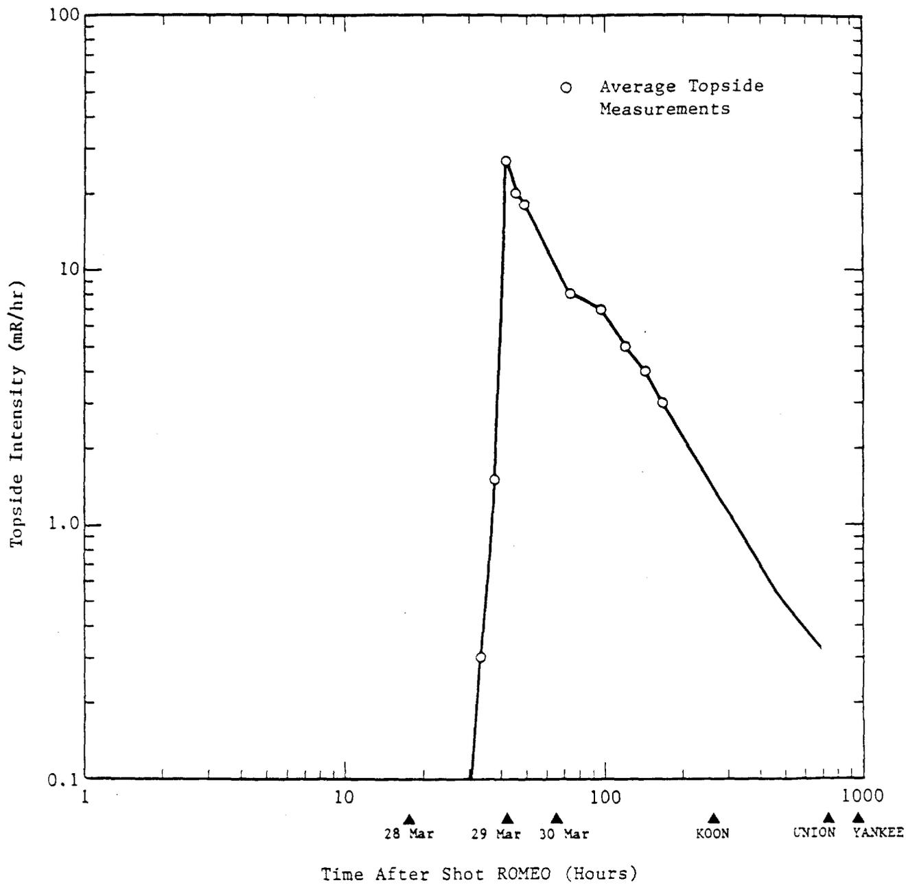
Figure 3.7. Topside intensity on USS MENDER (ARSD-2) following Shot ROMEO.
