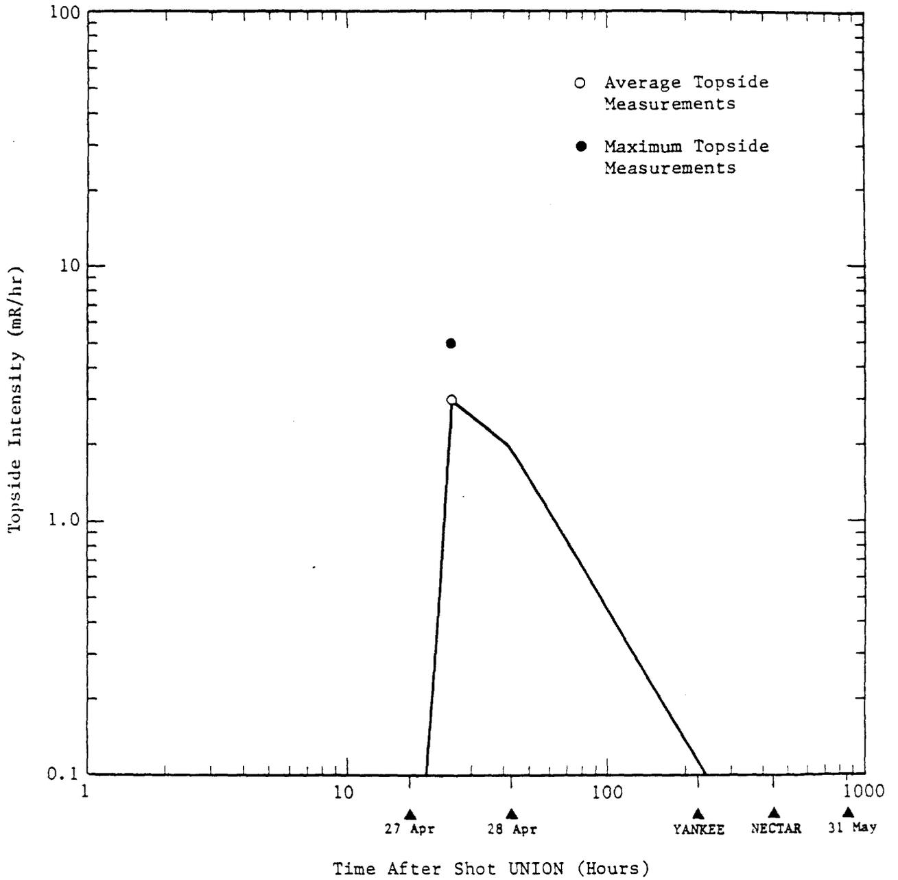
Figure 3.3. Topside intensity on USS SHEA (DM-30) following Shot UNION.
