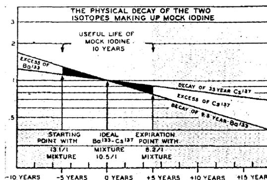
Fig. 3. The method of arriving at the useful life of mock-iodine
