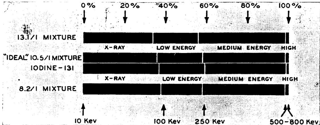
FIG. 4. The expected differences between iodine 131 and mock-iodine at the extremes of the accepted intercalibration mixture.
