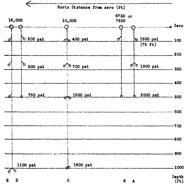
Instrument Line  ${}^mA^m$  is a 4-channel NOL system;  ${}^mB^m$ , a Hastings system;  ${}^mC^n$  is an 8-channel Wiancko system.
