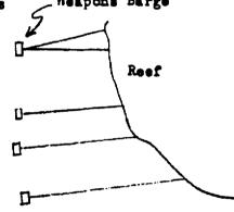
It is thought that a 1-1/2 chain should be sufficient to go from the moorings to the water. Then a 1/2" wire cable with breaking strength of 28,000 lbs will be adequate from the cable to the buoys. A deep sea moor will be put down to a 2800 lb anchor with a  $1-1/2^n$  chain leader. The instrument cans will be fastened to this system.
