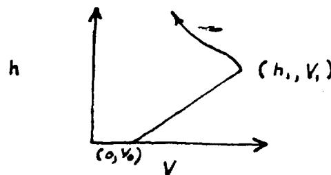
$$R = \frac{2 h_1 V_0 \tan \theta_0}{V_1 - V_0} \approx \frac{2 h_1 V_0 \theta_0}{V_1 - V_0} \quad 6)$$
