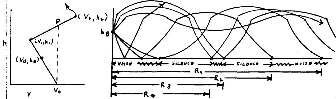
Rays with  $\cos^{-1} \frac{v_B}{v_0} \geq \theta_0 \geq -\cos^{-1} \frac{v_B}{v_0}$  are channeled and never strike the ground or travel higher than  $h_B$ .
