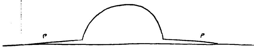
The precursor exerts a force normal to its surface (upward). This results in more damage than would be expected on moveable objects such as tanks.
