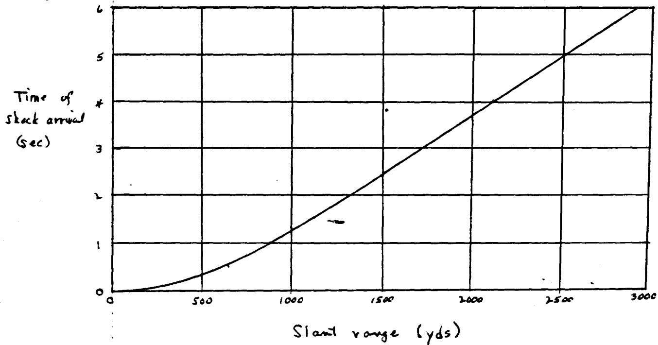
At shock wave breakaway time (about 15 ms,  $R=300$  ft) the shock wave velocity is about 15,000 ft per sec.
