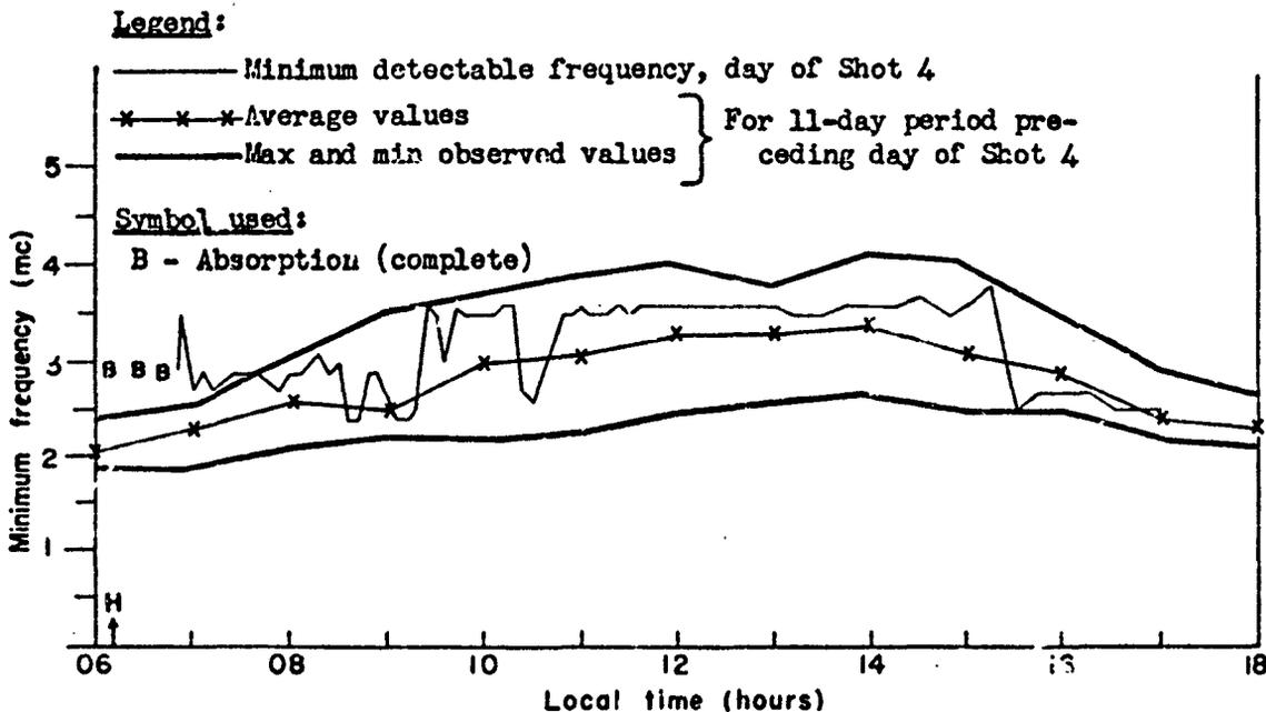
Fig. 3.1 - Minimum Frequency Detected at Rongerik for Day of Shot 4, Compared with Normal Values
