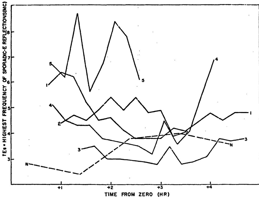
Fig. 3.3 - Highest Frequency of Sporadic-E Reflections at Rongerik following Shots 1 through 5, Compared with Normal Values.
