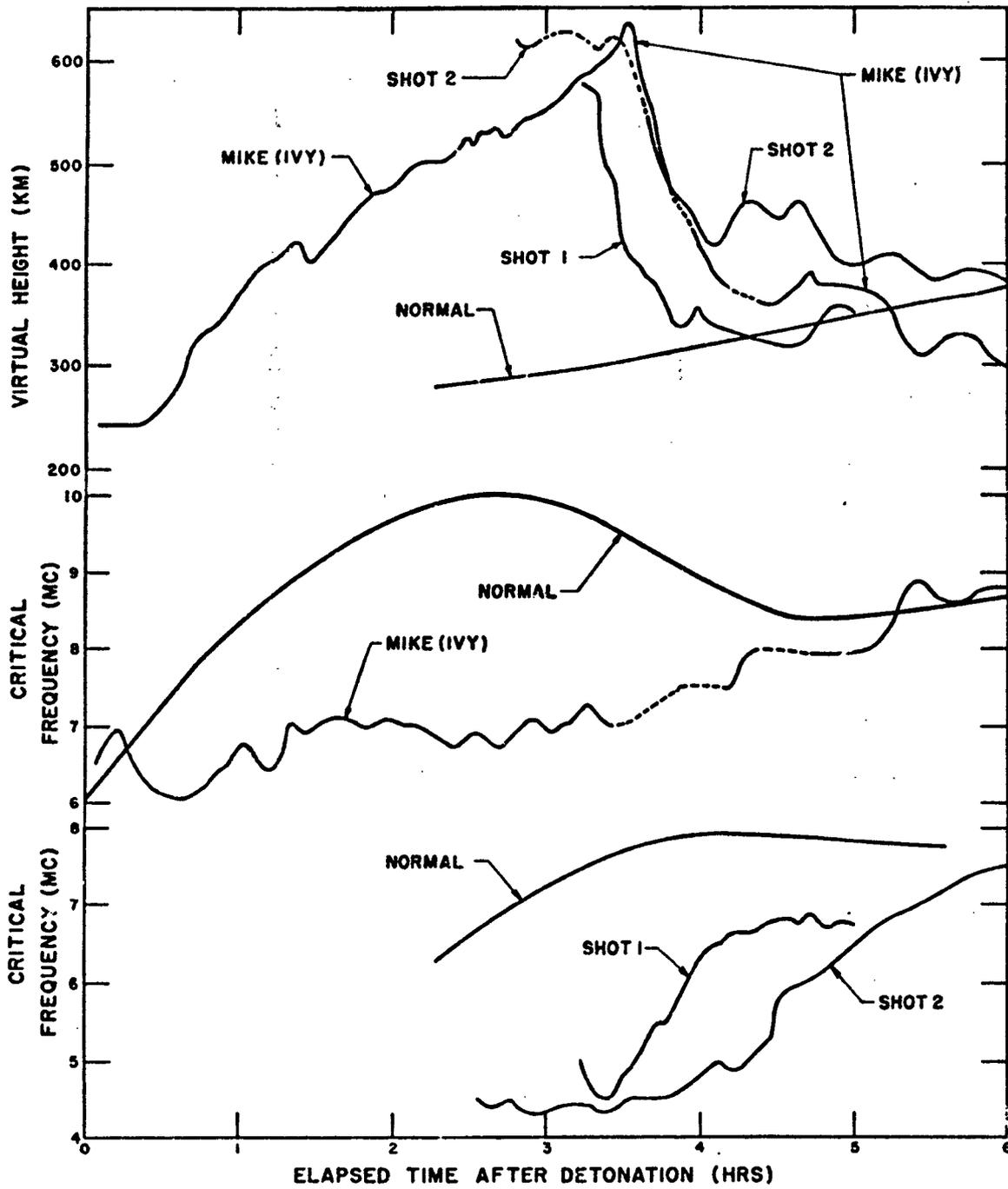
Fig. 3.9 - F2-Layer Virtual Height and Critical Frequency at Rongerik Following Shots 1 and 2 and at Bikini Following Mike Shot (Operation IVY), Compared with Normal Values
