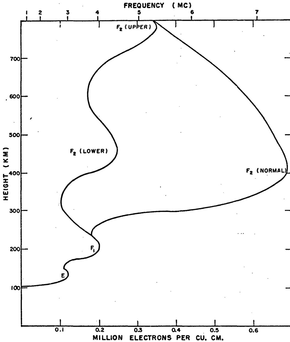
Fig. 3.12 - A Possible Electron-Density Distribution Above Rongerik at Shot 2 Plus 3 hr 49 min, Compared with a Hypothetical Normal Distribution
