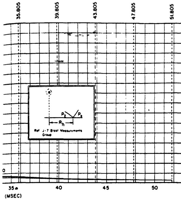
Pressure vs Time for Undisturbed Air at Several Horizontal Distances  $R_h$
