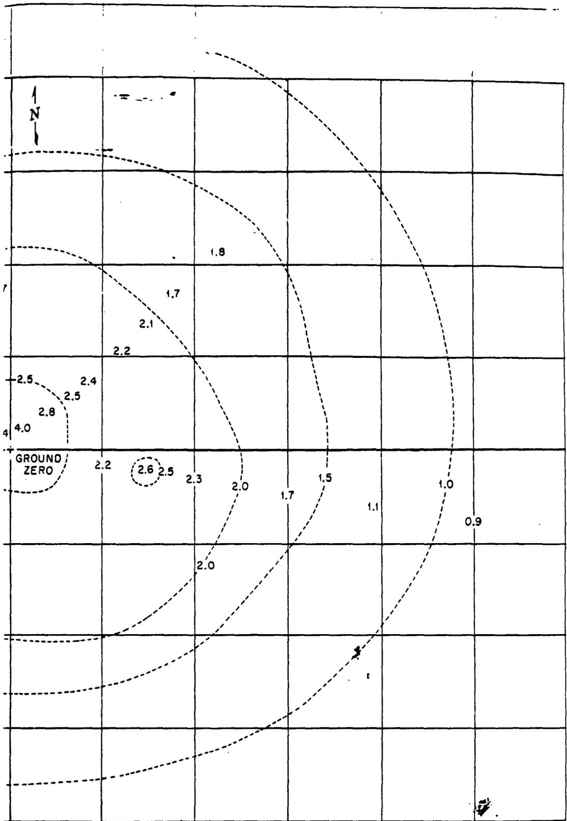
Contours represent changes in depth in feet. Grid lines are at 100-ft intervals.
