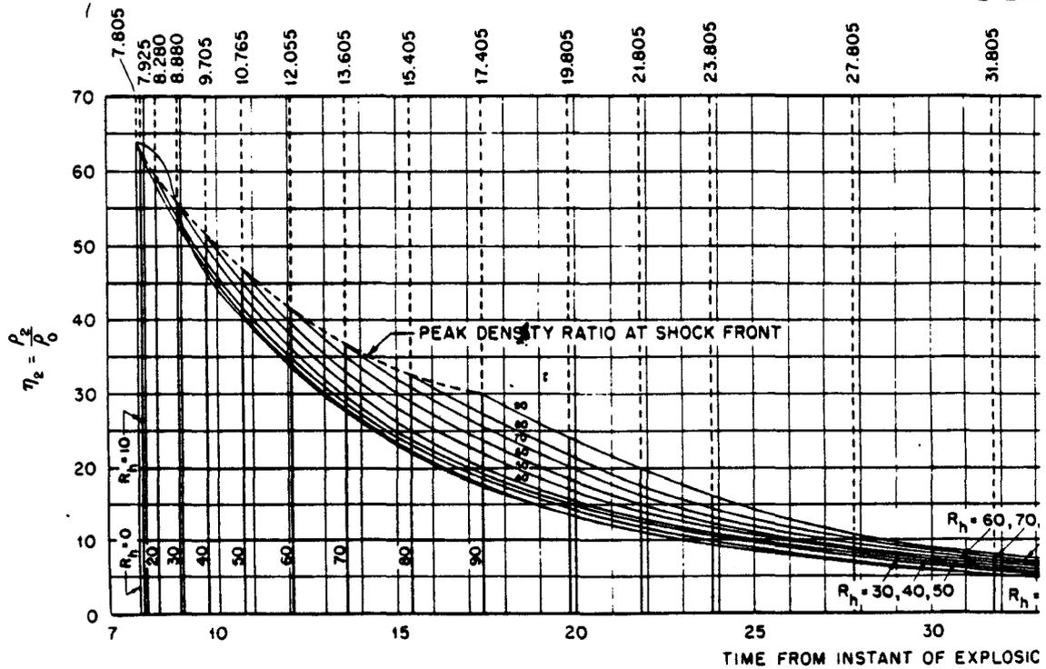
Fig. 1.3 Ratio of Air Density in Reflected Region on the Ground to Density Height of Burst, at Several Horizontal Dist
