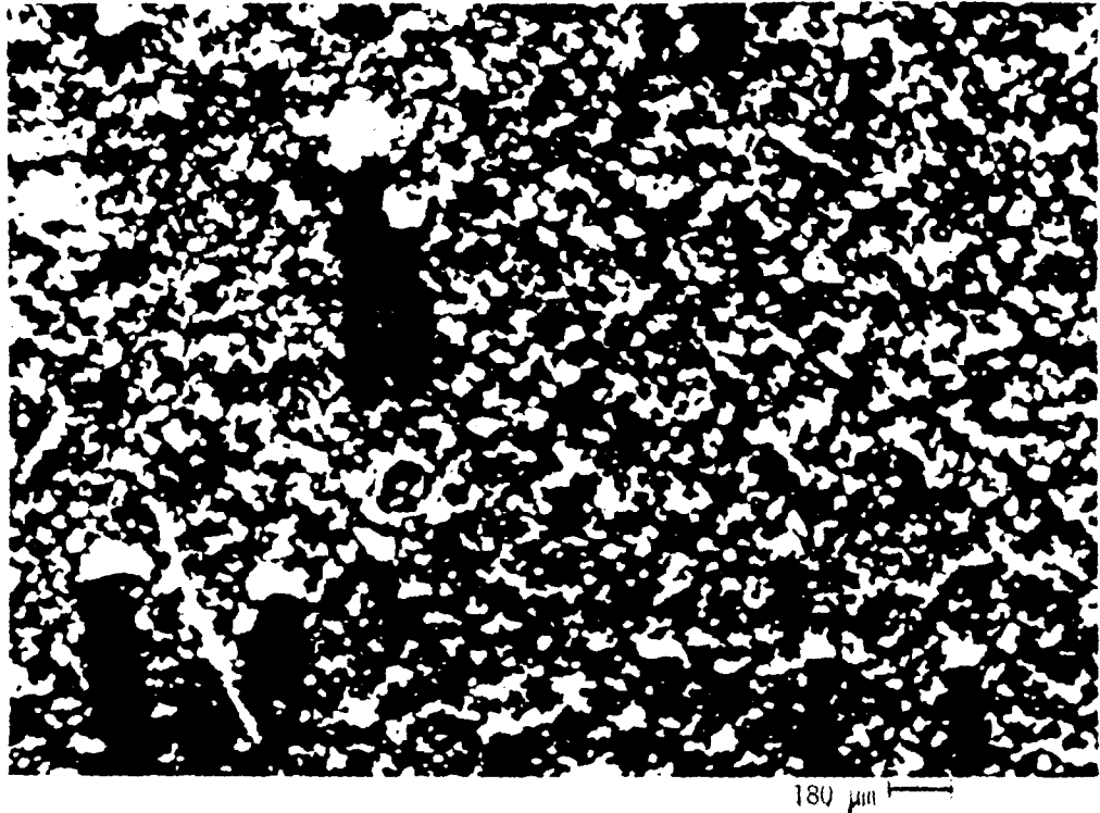
Figure 20. Reflected light photomicrograph of station B-20 surface sediment adhering to scotch tape. 20 X magnification. Many particles are agglomerates of the dried sediments.
