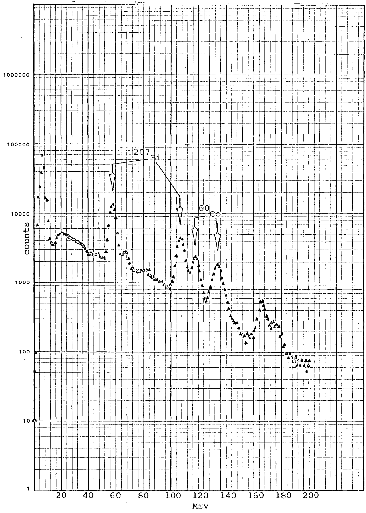
Fig. 1. Gamma-ray spectrum of sediment from Bravo Crater collected at a water depth of 160 feet, August, 1969.
