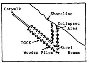
wooden piles was less structural than for the purpose of keeping boats from going under the dock. There is a steel waterline which is supported by the steel beams.
