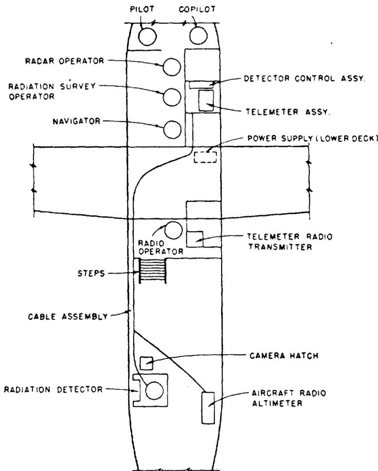
Figure 2.3 Radiation-survey-equipment mounting locations in P2V-5 aircraft.
