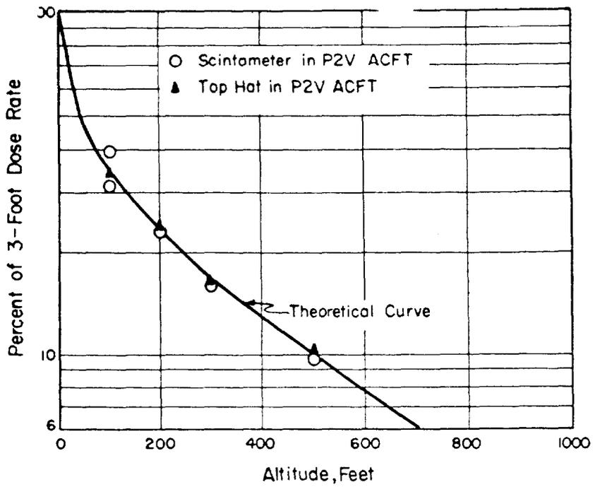
Figure 3.3 Radiation attenuation over land (P2V-5 aircraft).
