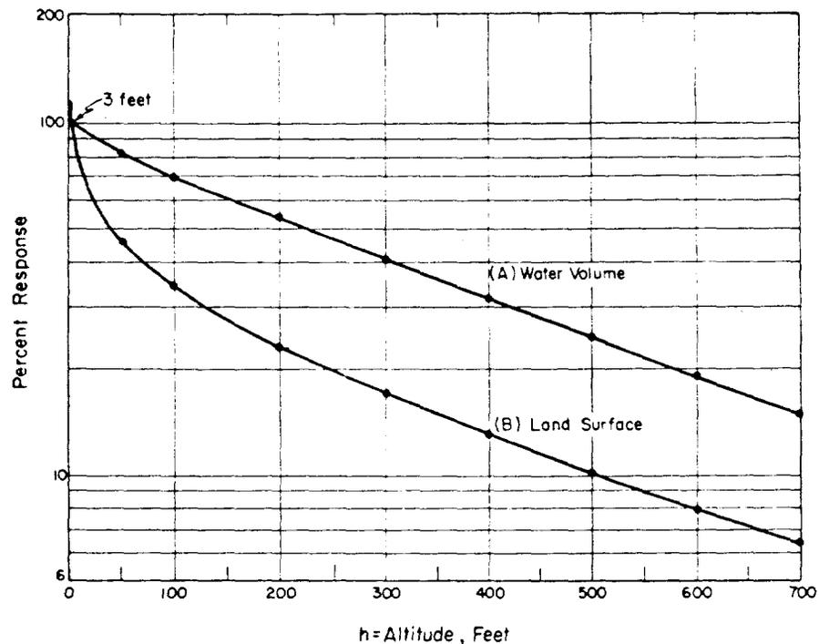
Figure 1.2 Radiation attenuation referred to  $h = 3$  feet.
