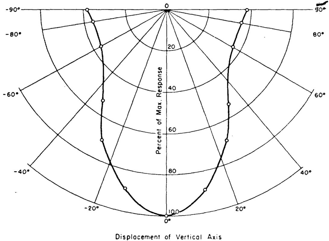
Figure 2.6 Angular response of Top Hat radiation detector, measured with 1-mg radium source. DOE ARCHIVES
