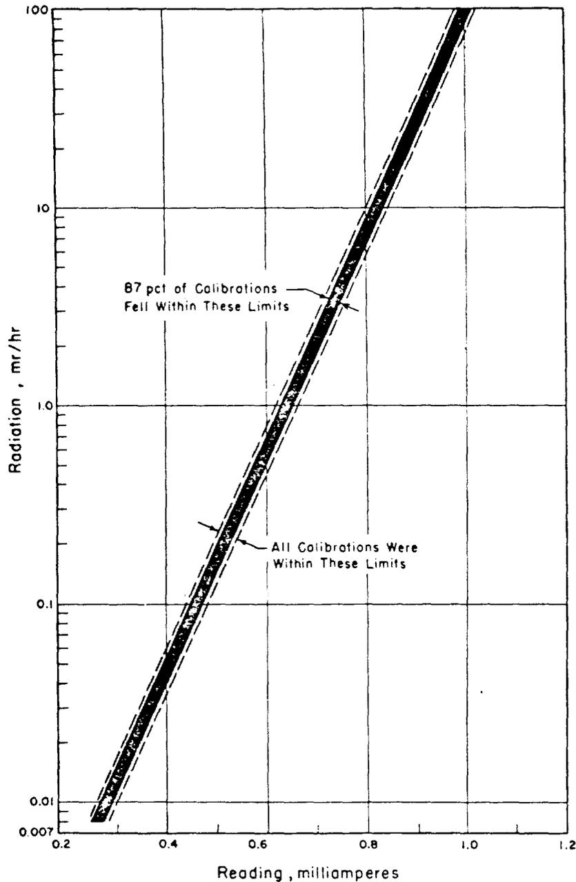
Figure 3.1 Summary of 37 pre- and postflight calibrations of Top Hat radiation detectors.
